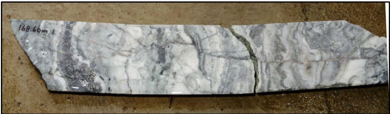
**Figure 7-9: Banded Low Sulphidation Epithermal Quartz Vein from Drill Hole RD10-009 (168.60 m).
