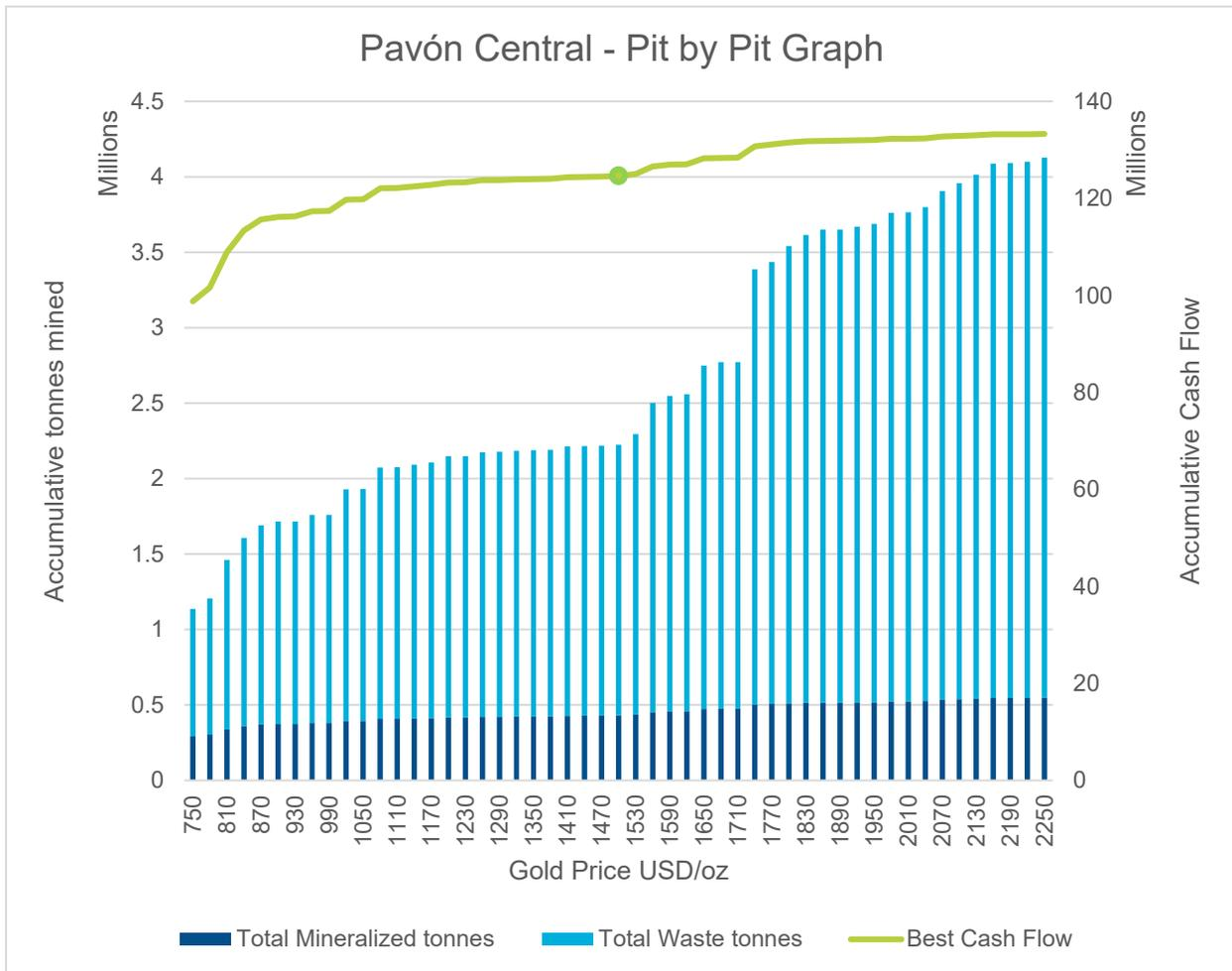
**Figure 16-8: Pavón Central Pit Optimization – Pit by Pit Graph**
