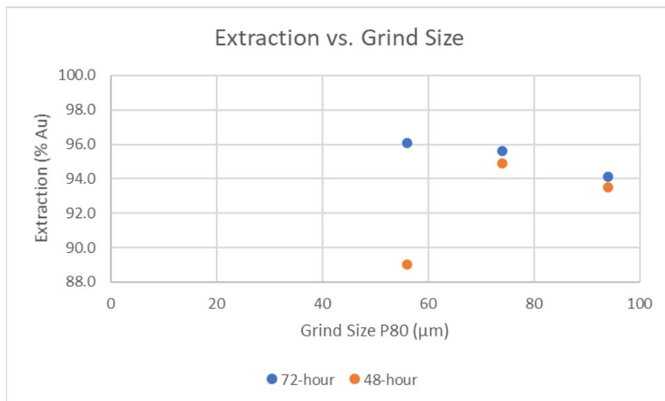
**Figure 13-3: Gold Extraction versus Grind Size after 72 Hours**
