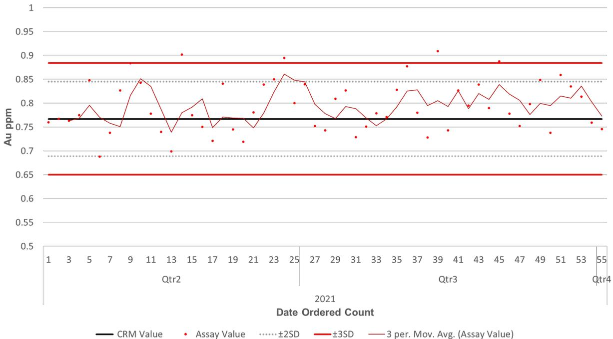
**Figure 11-39: Riscos de Oro Control Chart of SRM GSP6C (Gold)**
