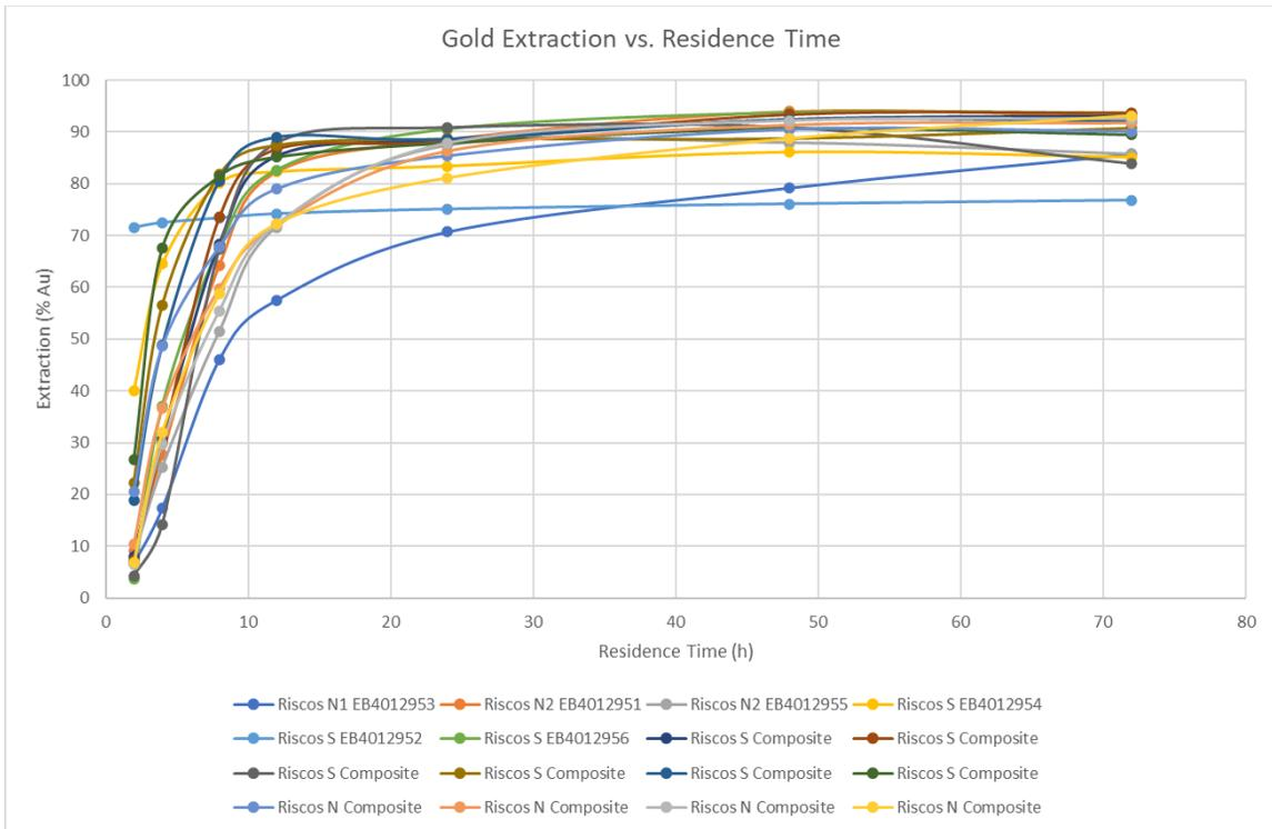
**Figure 13-15: PQ Core Kinetic Bottle Roll Test Gold Extraction**
