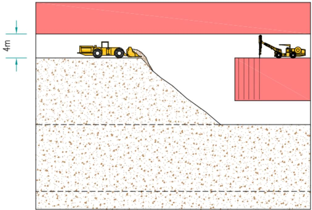
Figure 16-23: Avoca Method – Gap Left between Rock Pile and Bench
