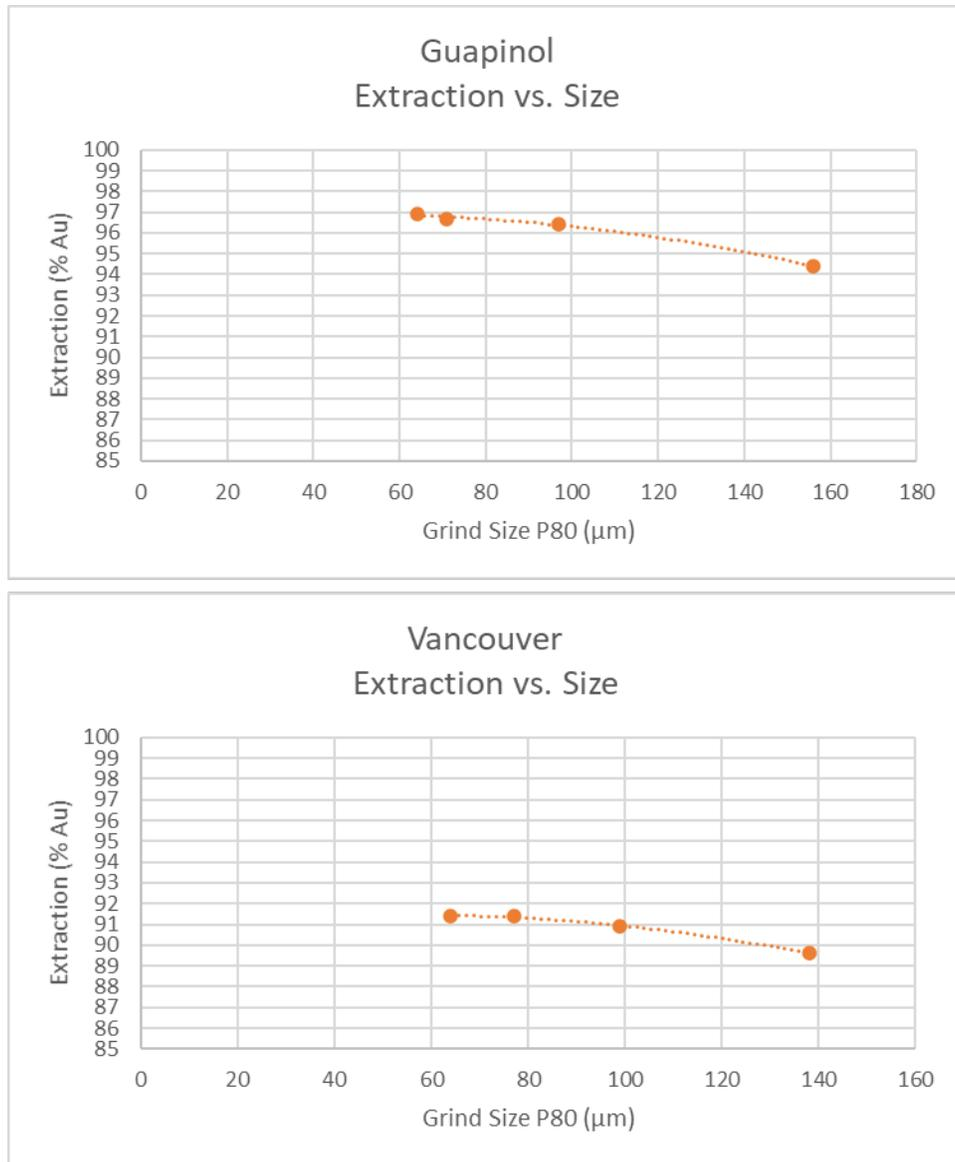
**Figure 13-10: PQ Core Composites 72-hour Gold Extraction and Grind Size**
