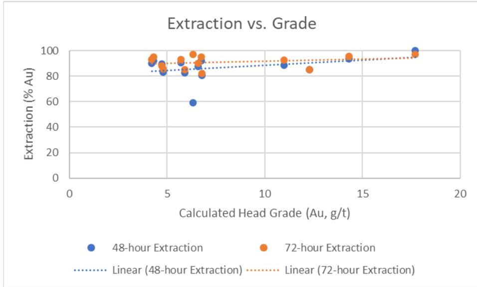
**Figure 13-18: Assay Reject Samples Extraction versus Head Grade**
