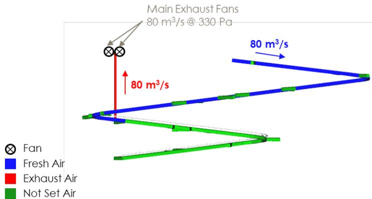
**Figure 16-33: Stage 1 – Initial Development, Ventilation Schematic**
