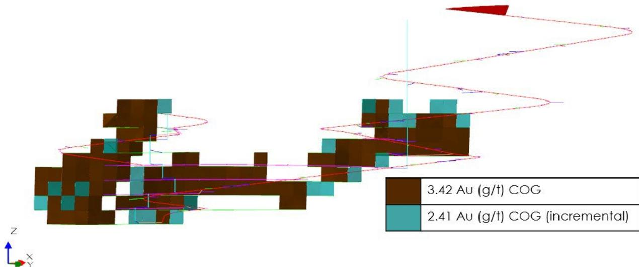
Figure 15-3: Long Section Showing Incremental Cut-off Grade Stopes
