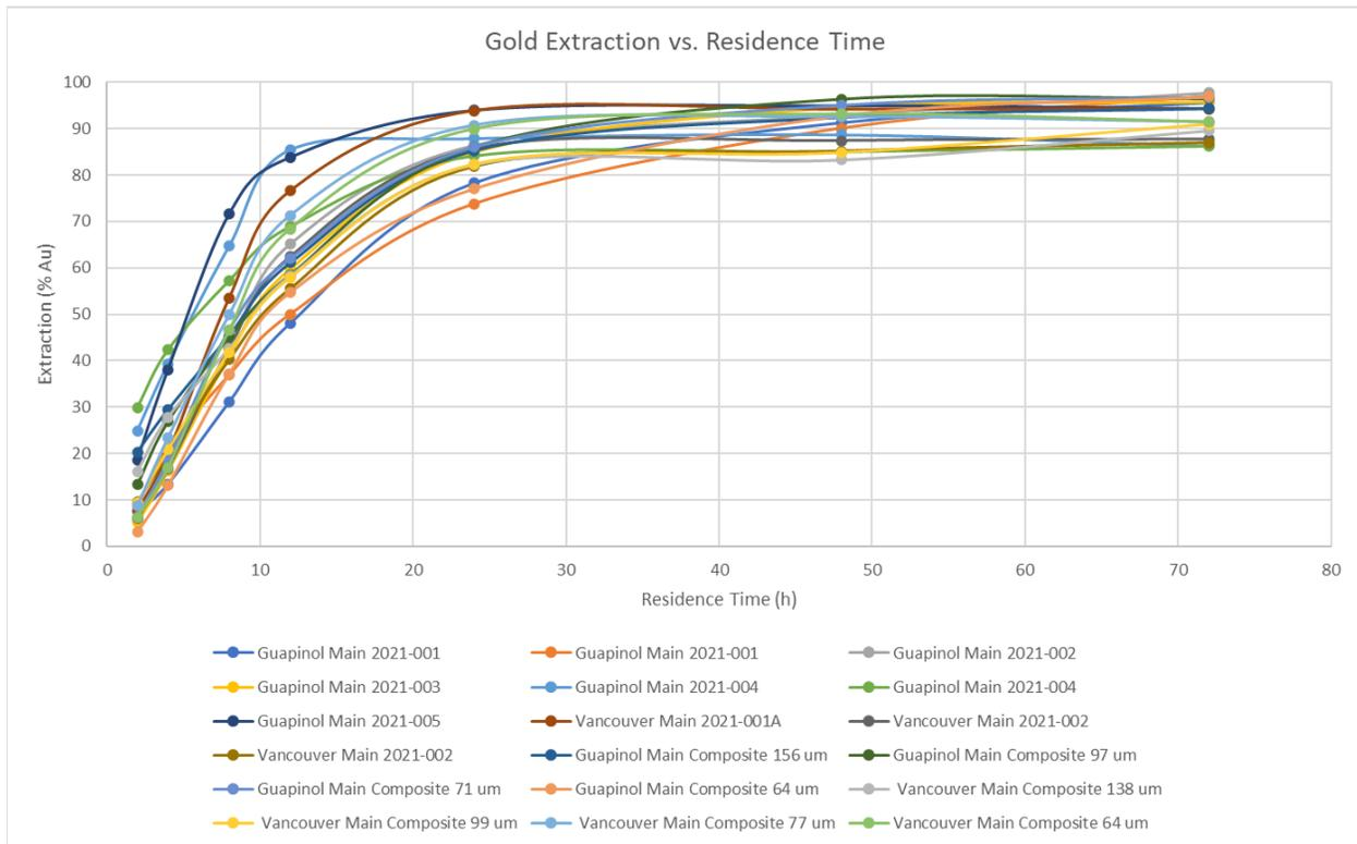
**Figure 13-8: PQ Core Kinetic Bottle Roll Test Gold Extraction**
