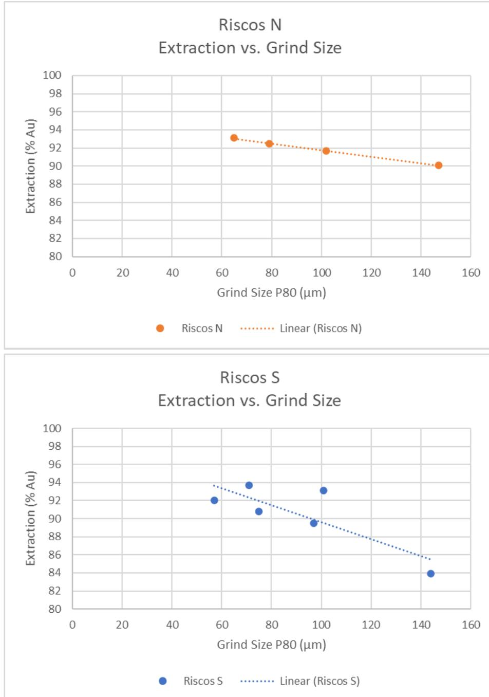
**Figure 13-17: PQ Core Composites 72-hour Gold Extraction and Grind Size**
