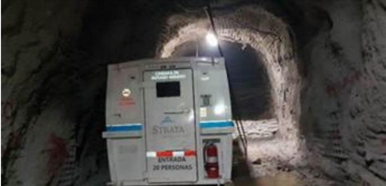
**Figure 16-26: Portable Mine-Rescue Refuge Station at Jabalí West UG**
