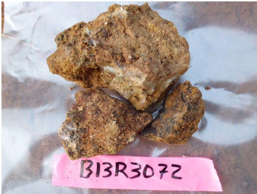
**Figure 9-3: Rock Samples B13R3072 with 14.2 g/t Au and 274 g/t Ag – La Sorpresa prospect, EBP**
