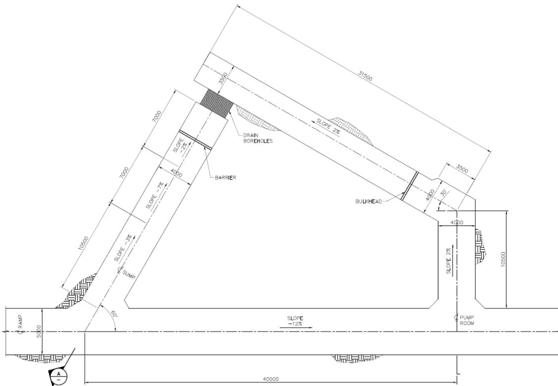
**Figure 16-36: Dewatering Pump Station**
