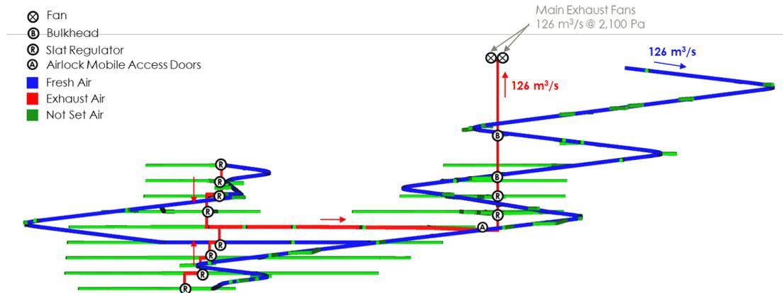
Figure 16-35: Stage 3 – Life of Mine, Ventilation Schematic
