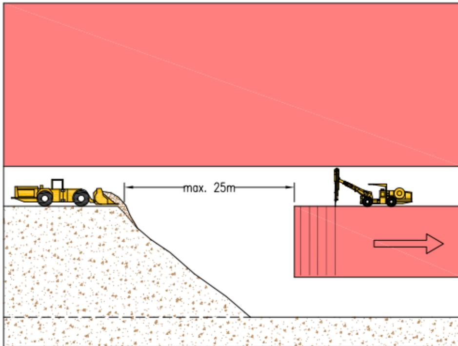
Figure 16-21: Avoca Method – Backfilling
