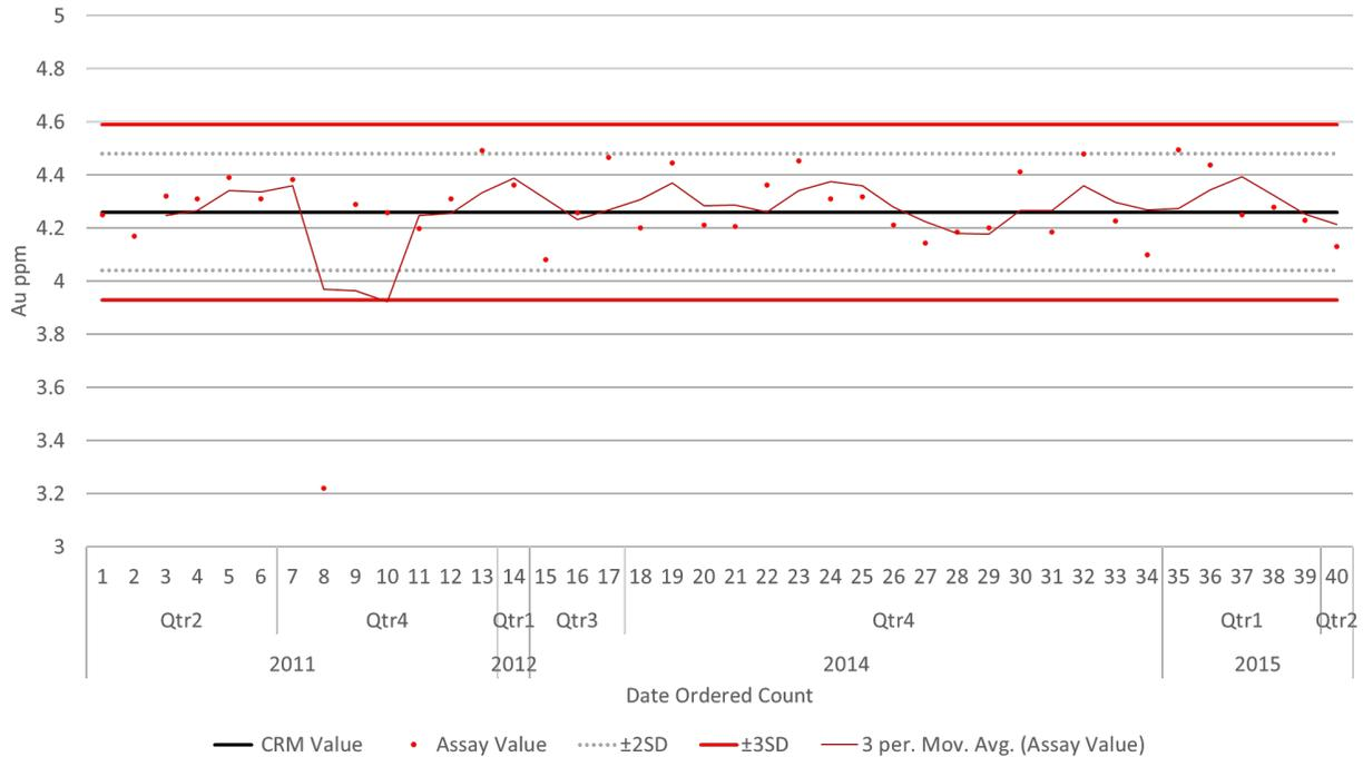
**Figure 11-38: Riscos de Oro Control Chart of SRM GS4C (Gold)**
