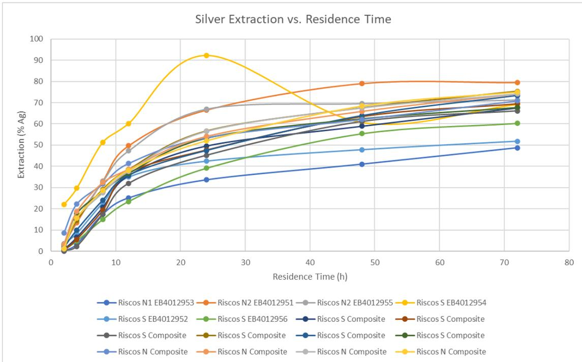
**Figure 13-16: PQ Core Kinetic Bottle Roll Test Silver Extraction**
