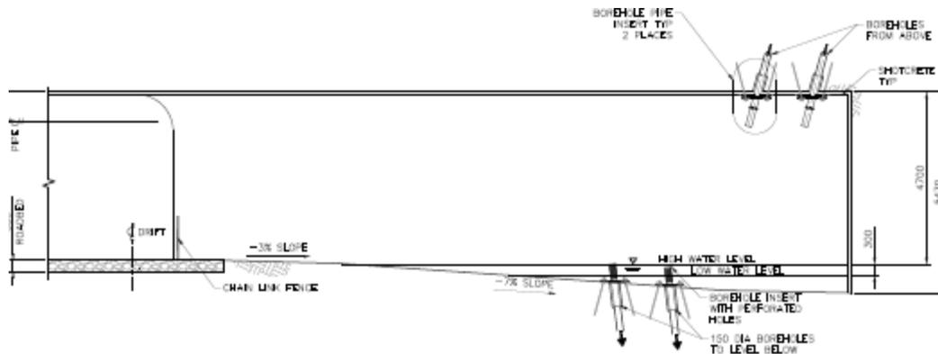
Figure 16-37: Borehole Sump
