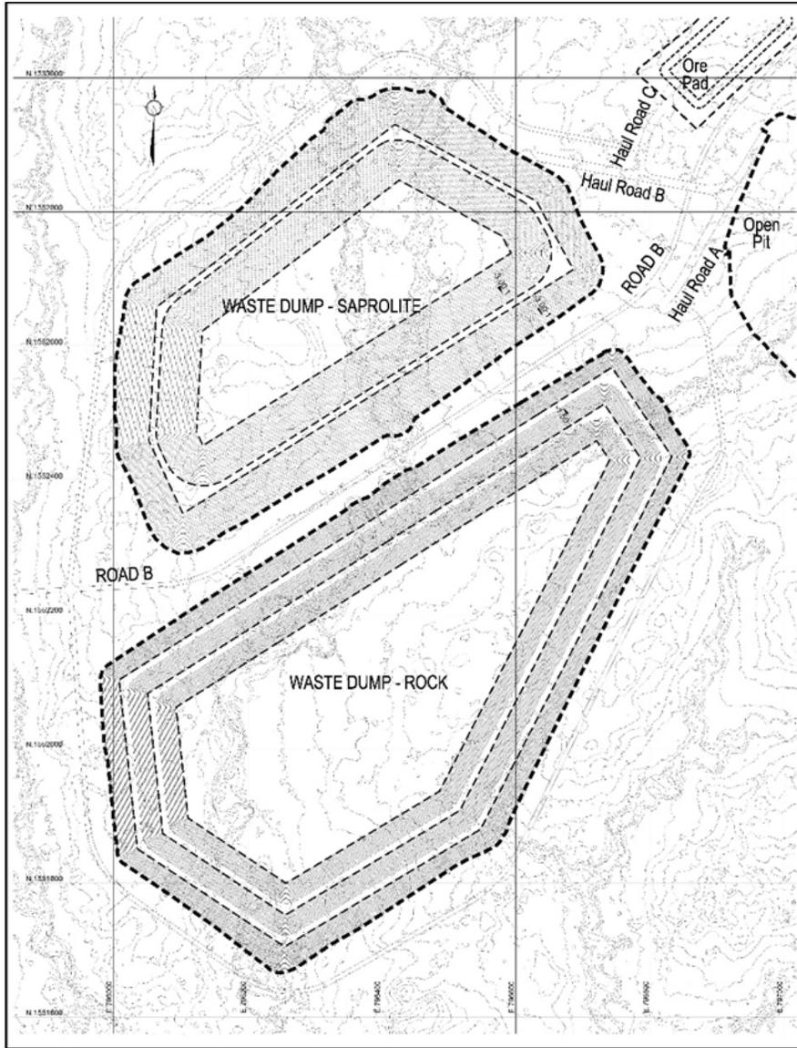
**Figure 16-14: Plan View – EBP-GV Dump Designs**
