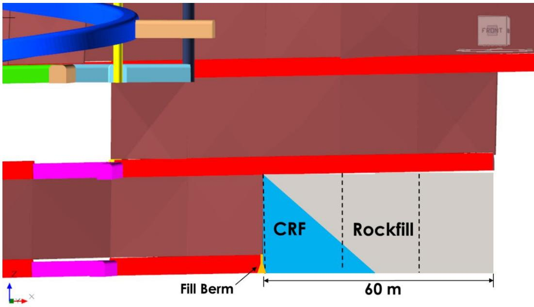
Figure 16-32: Stoping Block Backfill with Cemented Rock Fill and Rock Fill
