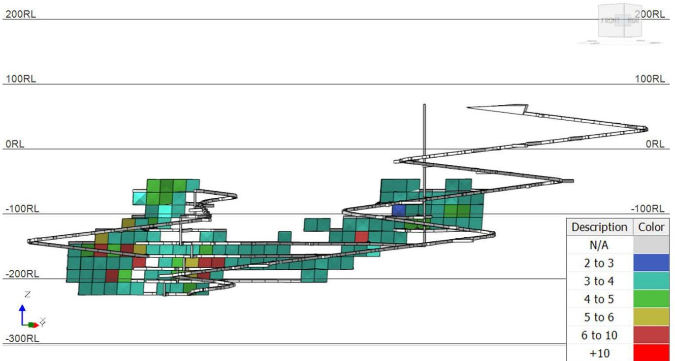
Figure 15-2: Long Section Showing Diluted Stope Widths
