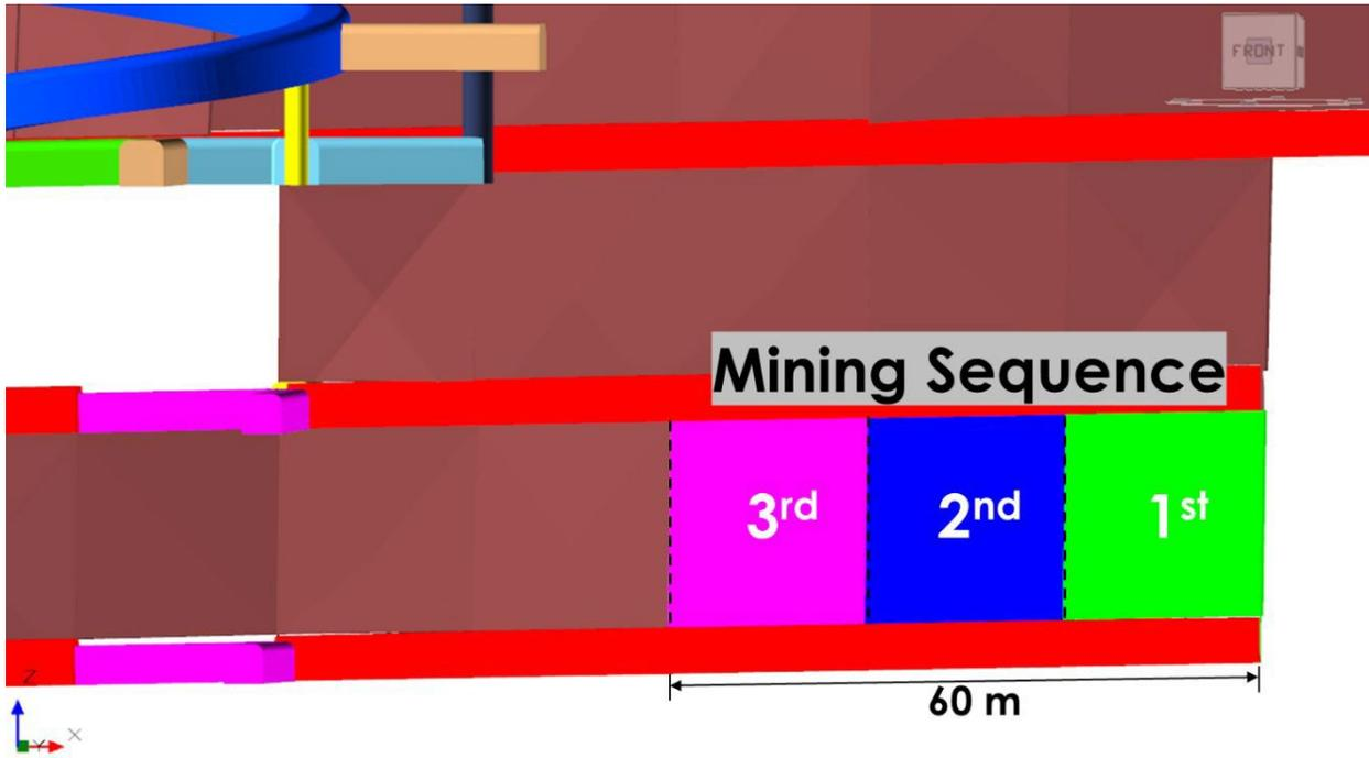
Figure 16-31: Mining Sequence Before Backfill for Longitudinal Retreat Stopes
