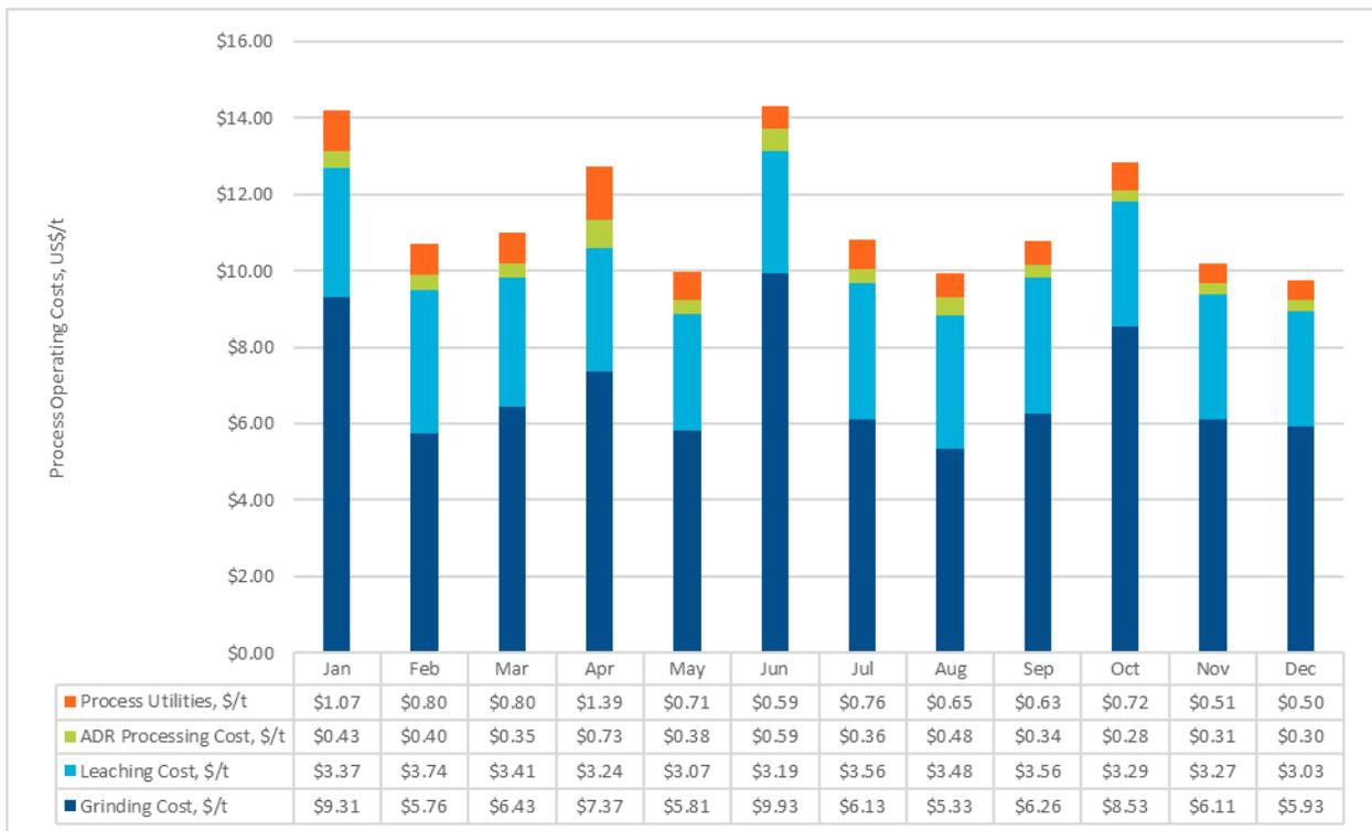
**Figure 17-6: Monthly La Libertad Significant Process Operating Costs for 2021**
