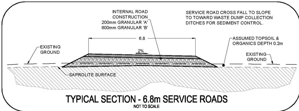
Figure 18-10: EBP-GV Typical Section – Service Road
