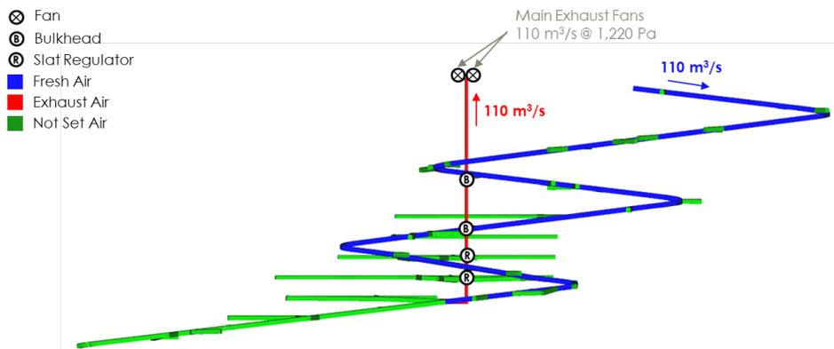
**Figure 16-34: Stage 2 – Full Production, Ventilation Schematic**
