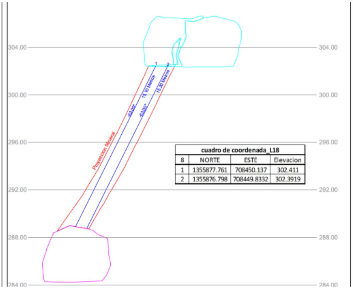
Figure 16-18: Avoca Drilling Layout - Section
