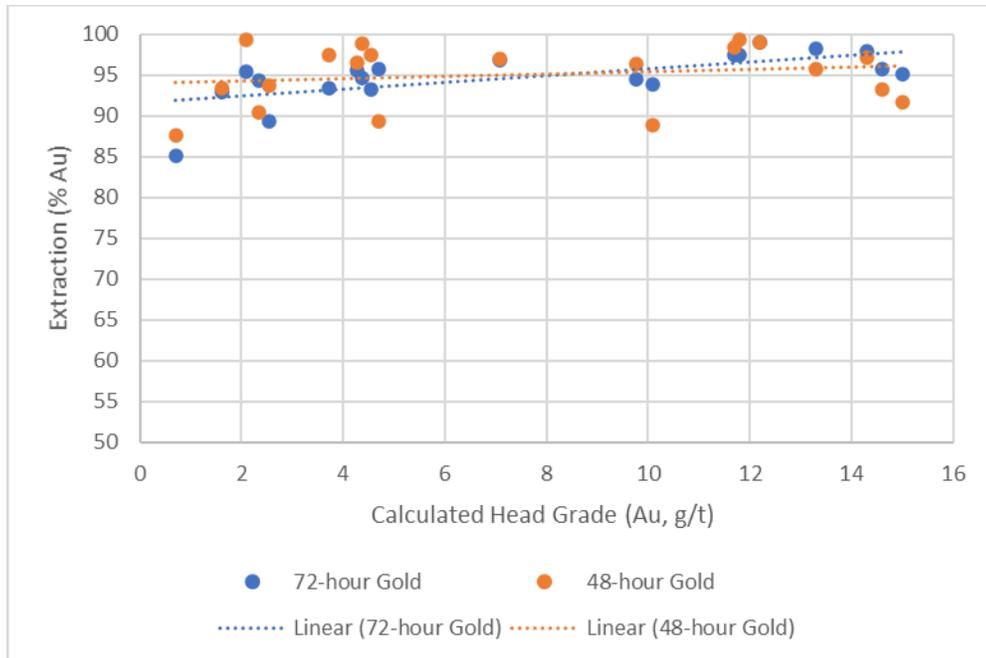
**Figure 13-11: Assay Reject Samples Extraction versus Head Grade**
