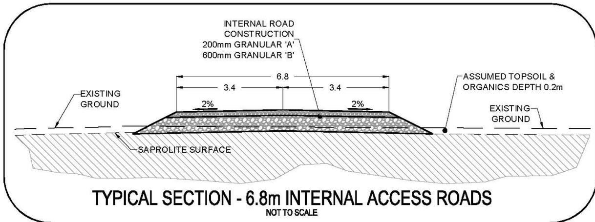
Figure 18-9: EBP-GV Typical Section – Internal Road
