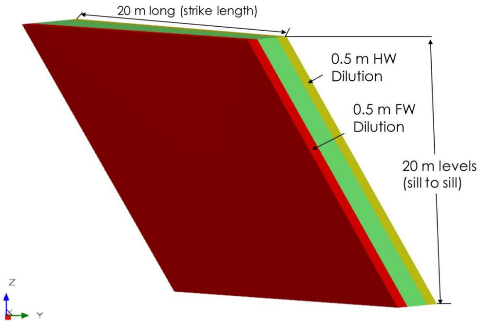
Figure 15-1: Stope Showing Dilution
