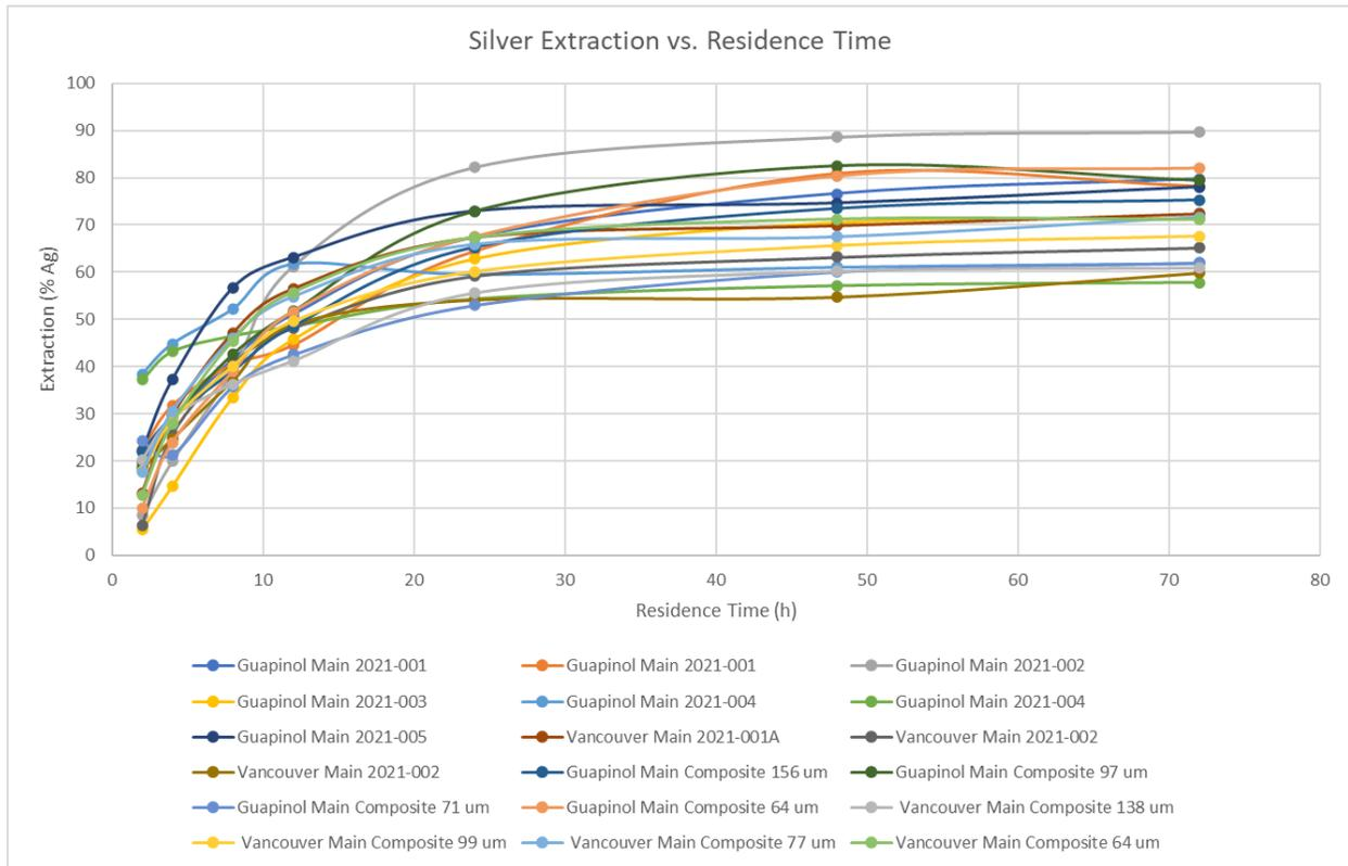
**Figure 13-9: PQ Core Kinetic Bottle Roll Test Silver Extraction**
